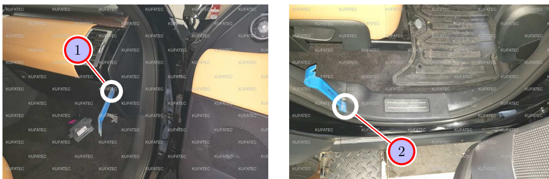
Figure 5: Removing trim panels passenger's side
